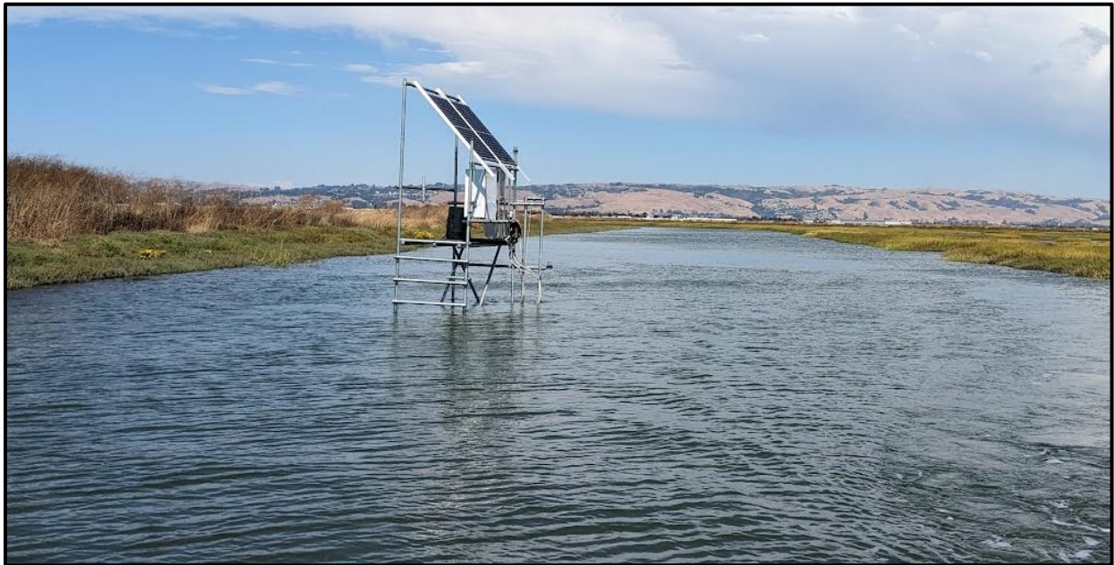
Figure 1. Instrumented platform in Mt. Eden Creek at the state of California's Eden Landing Ecological Reserve. Instrumentation installed on the platforms are measuring key sediment transport metrics to evaluate the delivery of sediment in the channel to connected saltmarshes. Funding for this research is provided by the USACE Dredging Operations and Environmental Research (DOER) Program.
