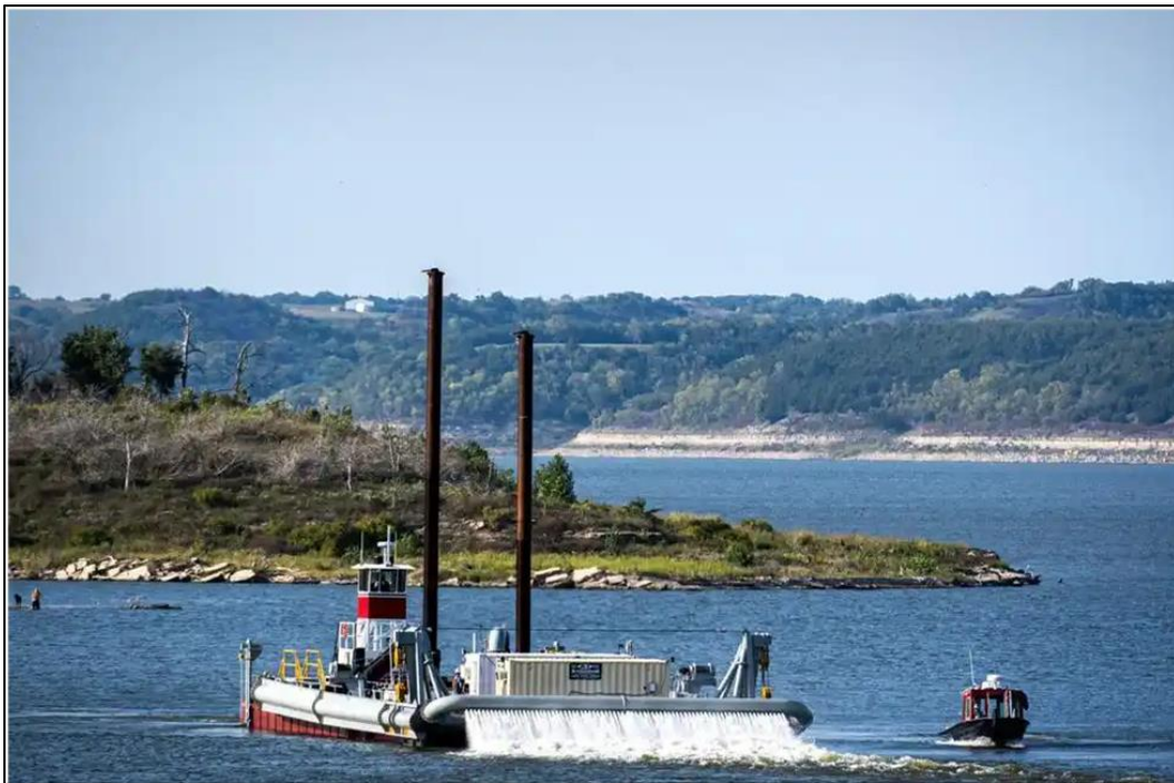
Figure 3. Dredge operating with jet-manifold above water [The Mercury].
