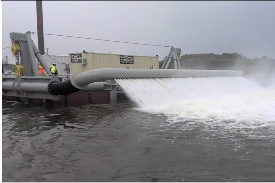
Figure 4. The jet-manifold with 78 x 2-inch nozzle configuration [Dredging Today].
