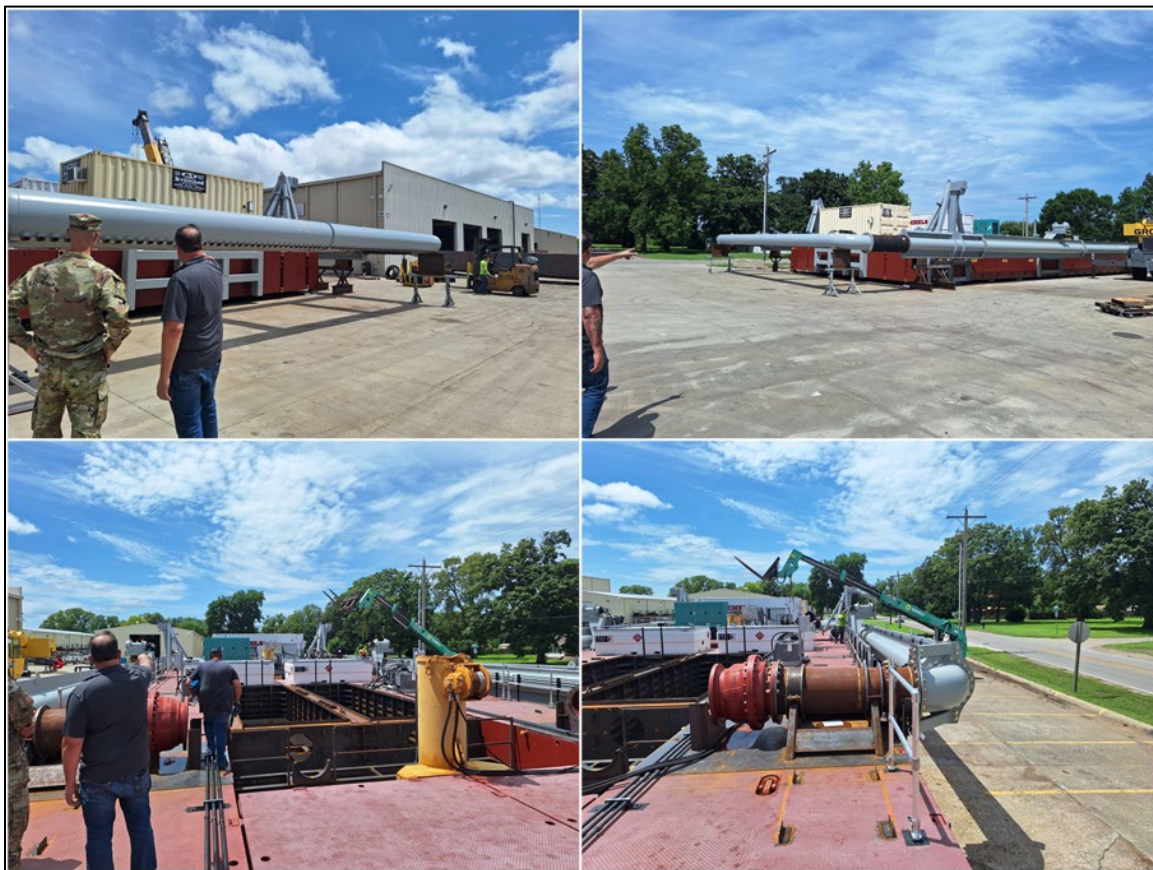
Figure 2. (Top Left) The injection manifold is 38' 11/16" ID edge-edge length with 78x total nozzles, each nozzle is adjustable for either 2" or 3 1/16" ID with 6" center to center jet spacing, also pictured is the push knee frame. (Top Right) The discharge pipe ladders are 100' - 24" steel pipe, with hoisting winches and gantry assemblies. (Bottom Left) Custom – Main Hull Sections instead of section barges are to support the pump set, parking spud well, and pump intake. (Bottom Right) Turning gland in the foreground and fuel cubes in background.
