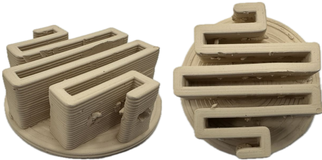
Figure 3. Photographs of the 3D-printed zeolite-clay composites used in the study.
