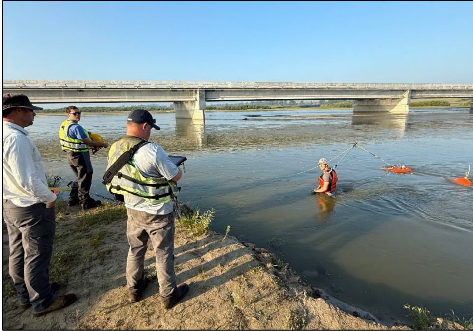
Figure 3. USGS and CHL staff collecting data near the 4-foot bedload sediment collector using an ADCP.
