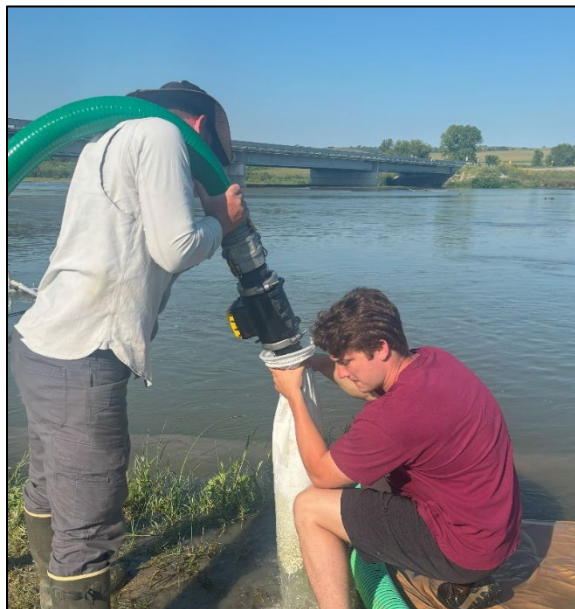
Figure 2. Sediment sampling using Millipore bags for gradation and capture rate measurements.
