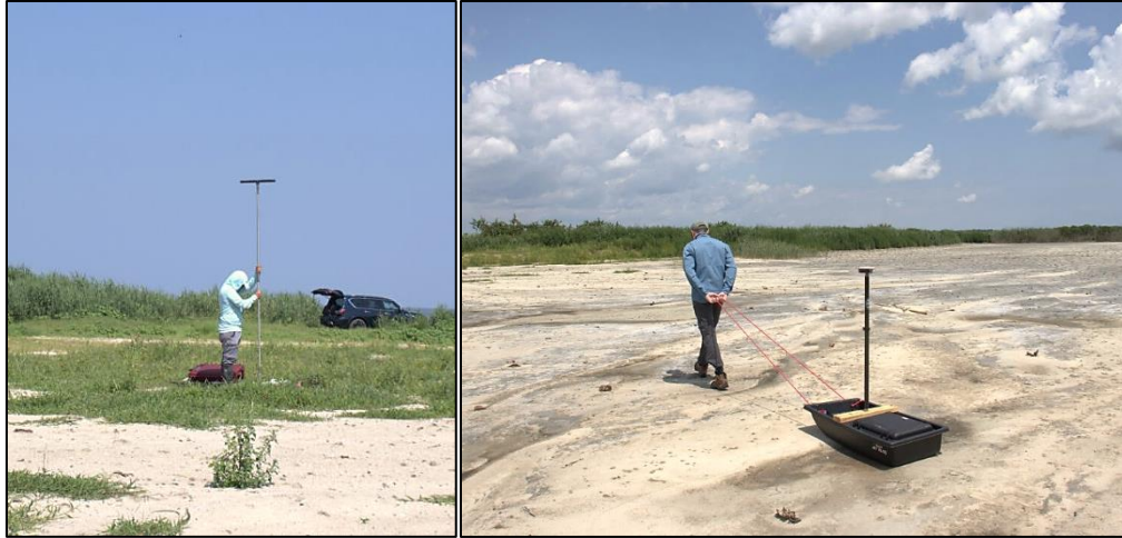
Figure 1. Daniel Gallegos (left) collecting auger samples and Shane Nichols-O'Neill (CHL ORISE Fellow) (right) pulling the GPR across a sand to mud transition zone within the CDF.
