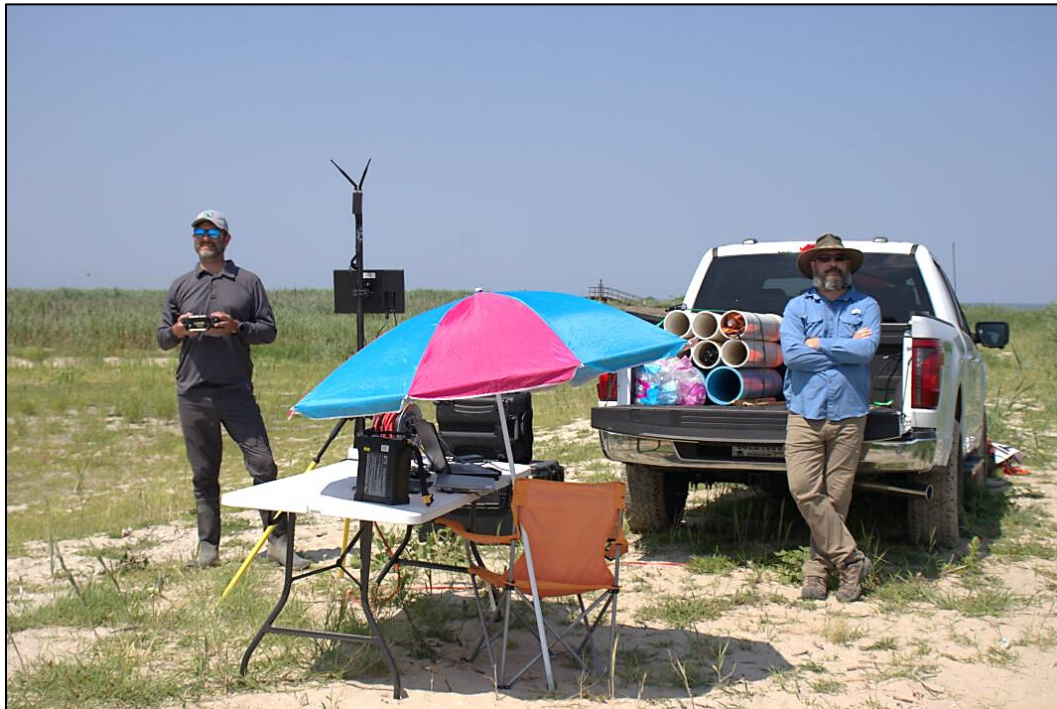
Figure 2. Heath Harwood (left) and David White (right), of JALBTCX, collecting uncrewed aerial system lidar and imagery data.
