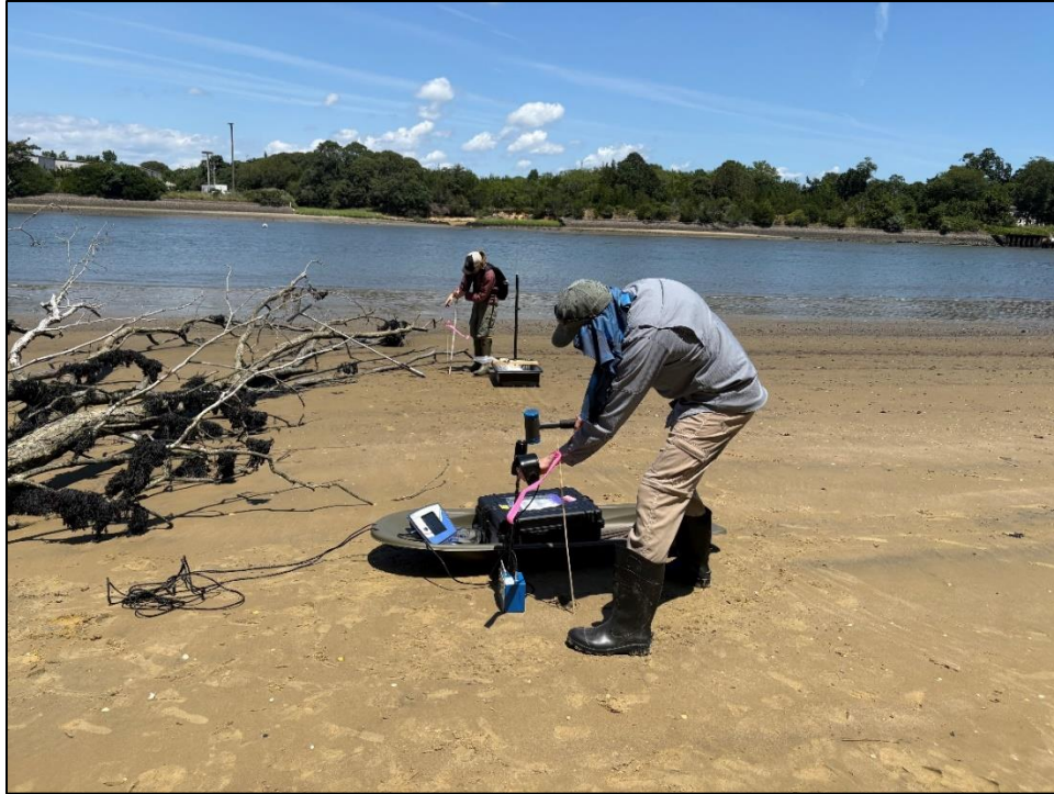
Figure 3. Shane Nichols-O'Neill (front) and Kathryn Smith (back) collecting a cross-section of DCP and hand auger samples at the proposed shoreline placement site.
