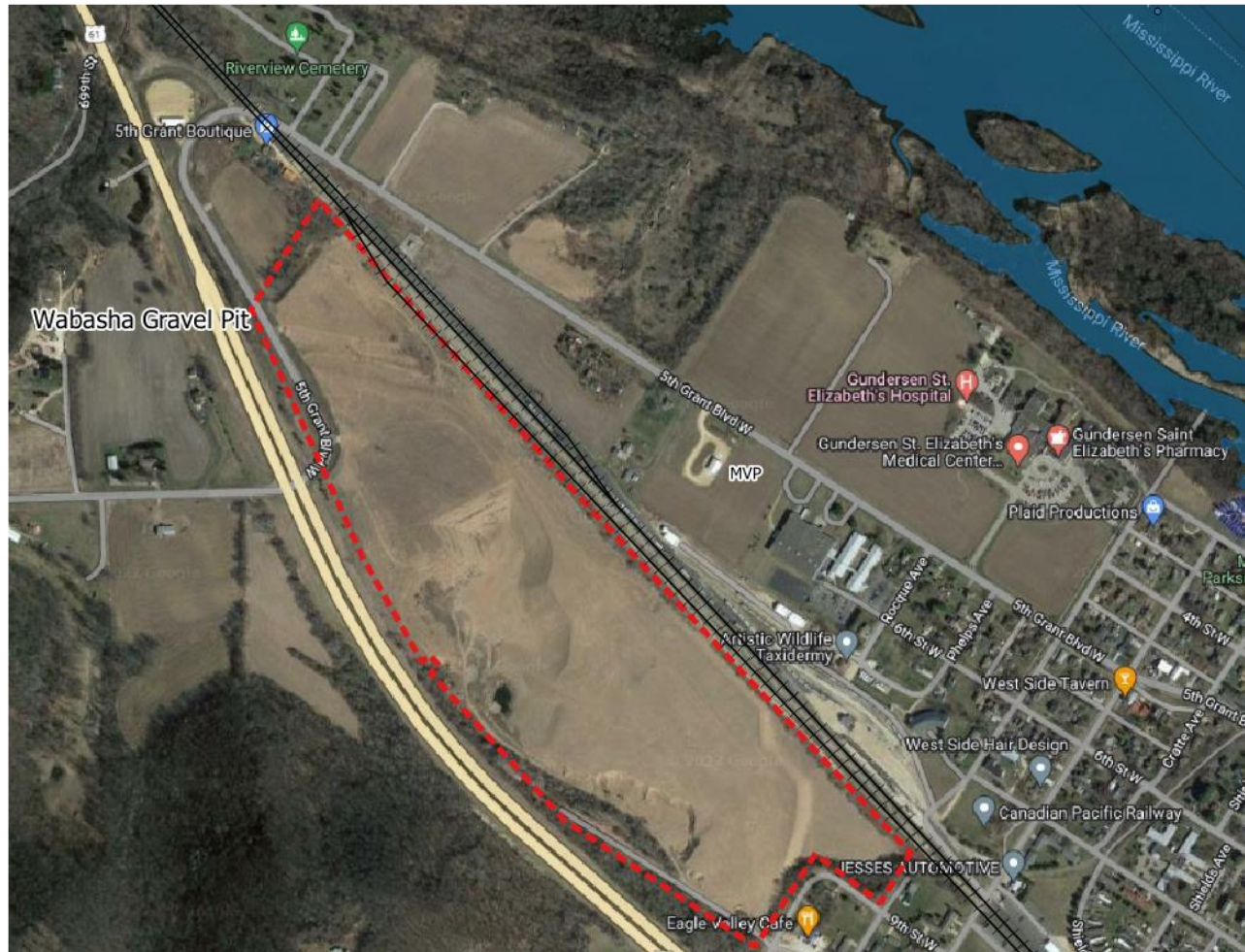
Figure 1. Mississippi River dredged sand stockpile at Wabasha, MN, is the result of dredging Chippewa River sand at a sand trap and along the navigation channel. A rail switching yard is adjacent to the 5 million cubic yard stockpile.
