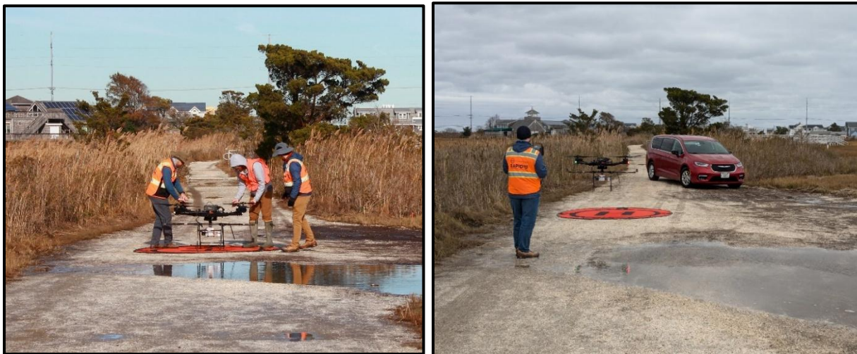
Figure 1. (Left) Initial set up. (Right) take-off of the Freefly Alta-X outfitted with the Phoenix Lidar Systems MiniRanger. From left to right are Dr. Michael Grilliot (RAPID), Dr. Brian Harris (CHL), and Andrew Lyda (RAPID). (Left photo taken by Devin Griffiths [TWI]).
