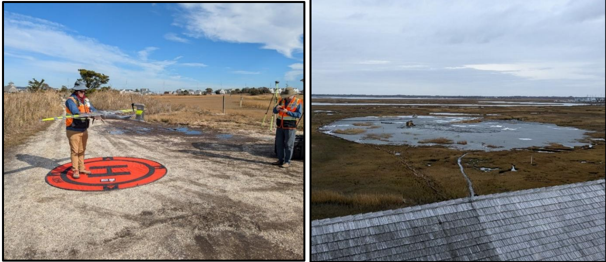
Figure 2. (Left) Calibration of the multispectral camera on the Quantum Systems Trinity Pro. (Right) View of the BUDM nourishment area from TWI's tower.
