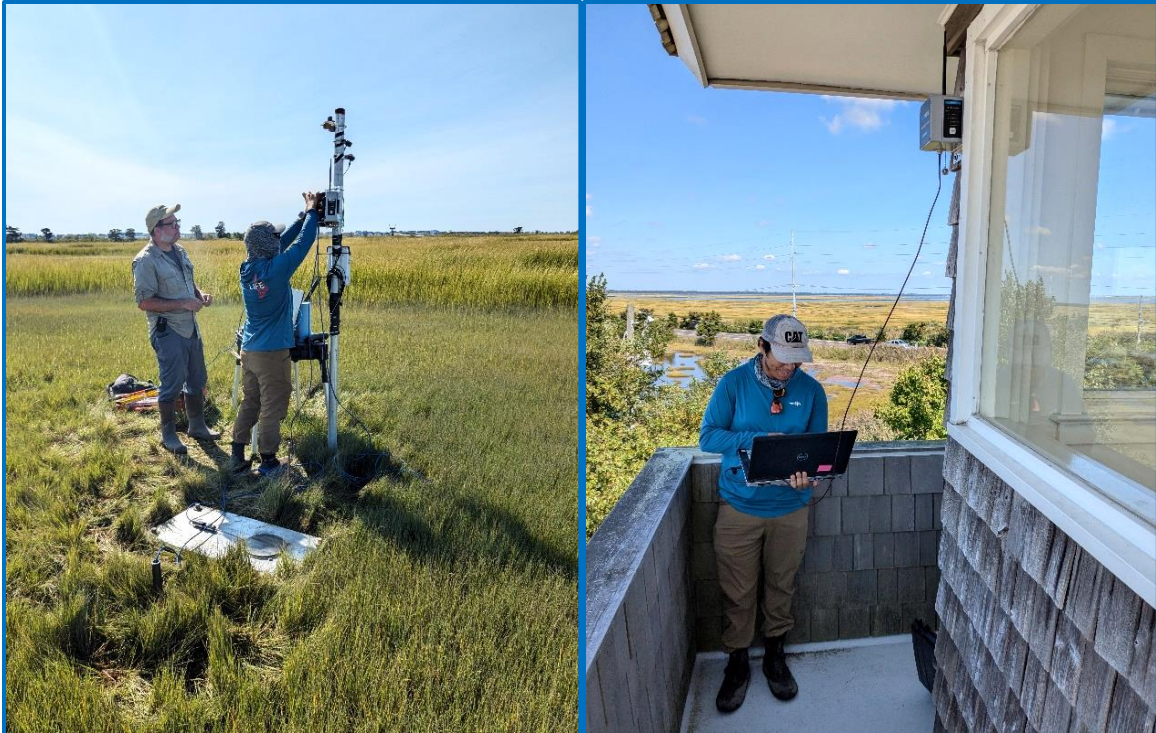
Figure 1. (Left) Installation of pressure cell and pore pressure sensors at the high-marsh site. From left to right are Dr. Anthony Priestas and Daniel Gallegos, both of CHL. (Right) Daniel Gallegos setting up the data transmitter on The Wetland Institute's tower. Photos collected by Dr. Brian Harris.
