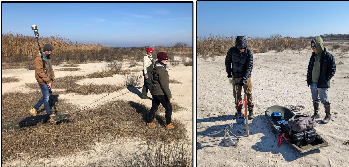
Figure 2. (Left) Ground penetrating radar (GPR) profile being performed by Dr. Kaitlyn McPherran (CHL), while real time kinematic (RTK) measurements were being simultaneously taken by Garret Albert and Nicole Ertle (NAP). (Right) Dynamic cone penetrometer (DCP) being performed by Dr. Jonathan Hubler (Villanova University) and Daniel Gallegos (LSU/CHL). Photos taken by Drs. Justin Shawler and Brian Harris (both from CHL).
