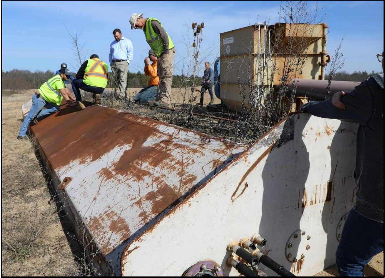
Figure 3. Lake Altoona District Board, Streamside, and ERDC inspect the 30-ft collector that ran for 3 years in the Cuyahoga River before being donated. We are standing on the collector, and the yellow box is the first step in a sand-water separating system that retains sediment in the placement site and returns water to the river.
