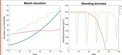
MEM model output for North Inlet, SC marsh comparing a baseline scenario to a TLP scenario in which 12-cm of sediment is added every 20 years starting at year 15.
