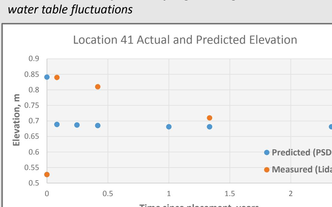
Surveys (RTK and/or lidar) were taken over time to evaluate the elevation change at various locations across the site.
