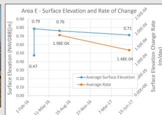
Terrestrial Lidar and elevation data sets are being used to analyze the elevation change (consolidation) over time. Preliminary results at one location (Area E) shows moderate elevation change which may be attributed to consolidation, dredge material surficial equilibration.
