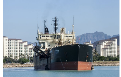
The trailing suction hopper dredge Essayons is used by POH to keep Federal navigation channels open in Hawaii ports.
